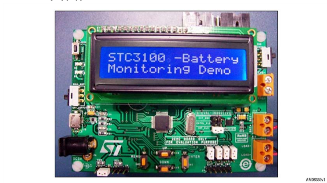
Figure 1. STEVAL-ISB011V1 Li-Ion battery monitor and gas gauge based on STC3100
